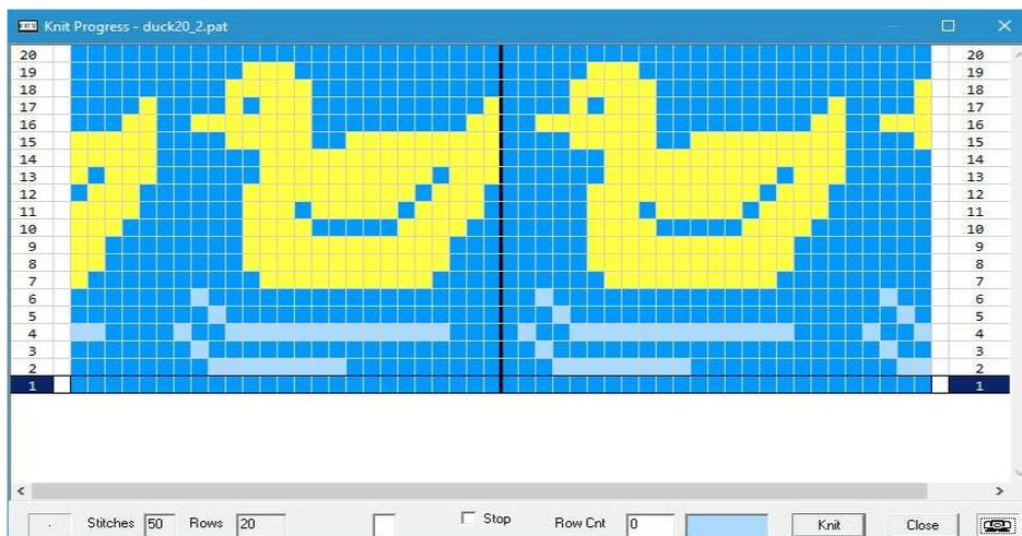
Your computer screen displays the stitches to be knitted and the progress of your knitting. You can select with a single click the row where you want to start knitting. The full screen of your computer can be used to display your pattern as it will be knitted. A row counter, carriage position and contrast color indication are displayed too.
